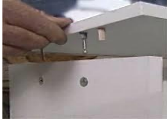
Fig. 5 Fixing screw and locking cam
