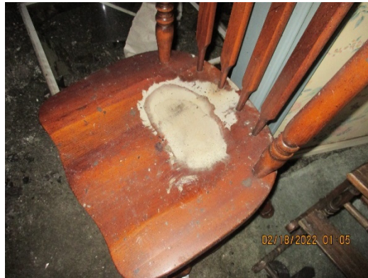
Figure 7: Blushing on Wood Finish
